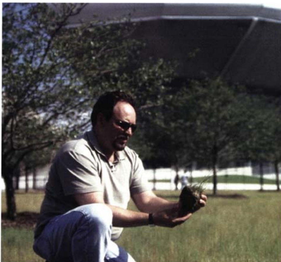
Bruce inspects a core sample of one of nine soils his firm engineered specifically for Chicago's Museum Campus.
